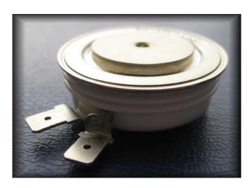
IXYS UK Westcode Ltd. has introduced a 500A, 2.5KV GTO (gate turn-off) thyristor in a new smaller package. The new GTO thyristor rated at 500A & 2.5kV is based on IXYS UK's established S500KC device; the die design has the same active area performance, but with an improved termination design which allows the device to be encapsulated in a smaller 25mm pole face package.
