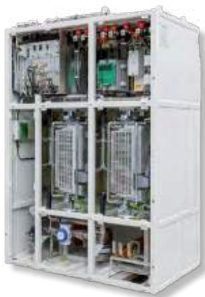
KONTRAC GP550AC propulsion converter for EMUs
