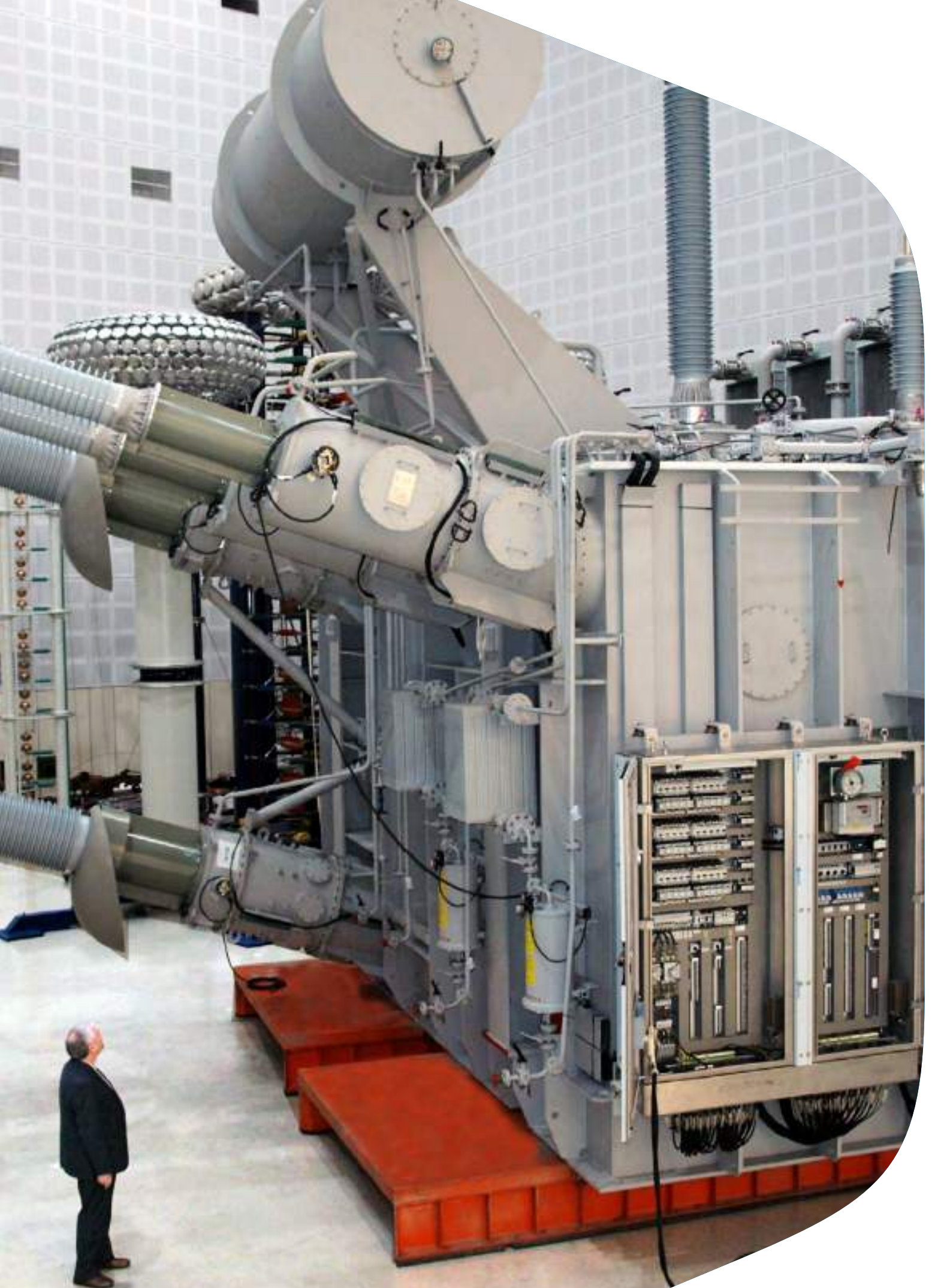
HVDC converter transformer delivered to New Zealand
