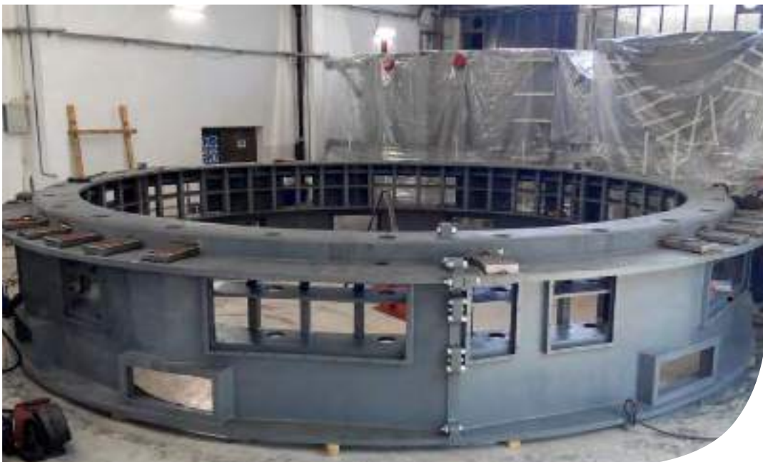
Hydro-generator – stator frame
