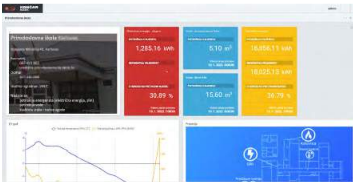
MARS used for energy efficiency of school building
